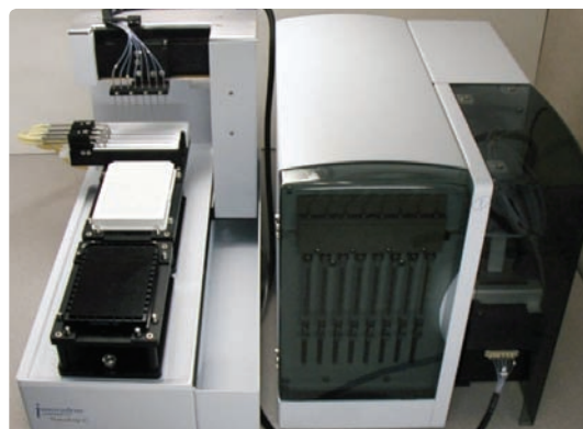
Picture 1 — Innovadyne Nanodrop non-contact low-volume liquid handler (IDEX health and Science, LLC)
