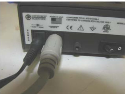
Figure 4: Power and communication connections to the Nano Flow Sensor.
