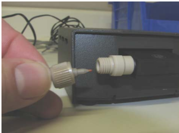
Figure 5: Fluidic connections to the Nano Flow Sensor
